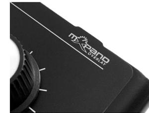
It is possible to remove the overlays and reapply them at any time. To do this, there are 2 tiny "tabs" at the top where the overlay is lifted (near the volume and the cutoff knob).
