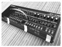
**Attention:** The adhesive strips (for temporary fixation) must **not come loose** during this time! In addition, make sure that the now-adhesive overlay does **not** touch the device in this step.
